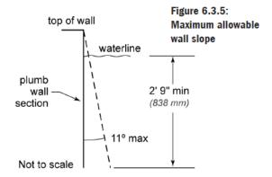
**6.3.5 Walls.** Where walls join the floor the transitional point or profile shall comply with the following:
