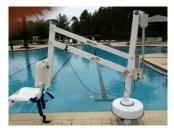
If the lift is an Extended Reach (as shown above), first check to be sure all connections are secure. Check extension cable for damaged or pinched area. Plug hand controller directly into control box. Does the hand controller work? If yes, the extension cable needs to be replaced.
