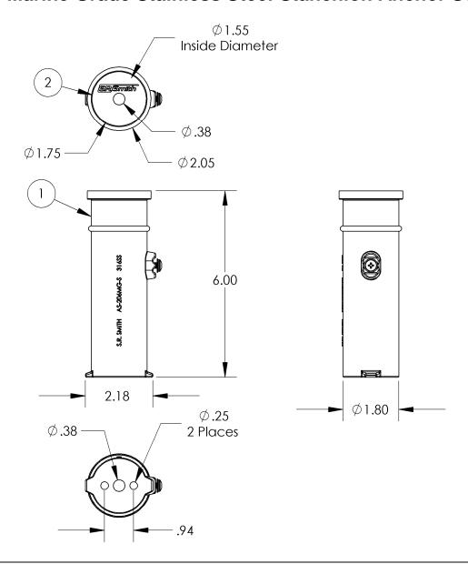
**Specification:** The 1.5" Marine Grade Stainless Steel Stanchion Anchor Socket (Item 1) is made of 316 stainless steel and is 6" (152.4mm) deep, allowing for mounting 1.50" O.D. (38mm) fixtures without the use of a wedge assembly. The anchor is tapped for the provided #10 UNC brass grounding screw. A marine grade stainless steel cap (Item 2) is provided to mount flush with the deck when the fixture is removed.
