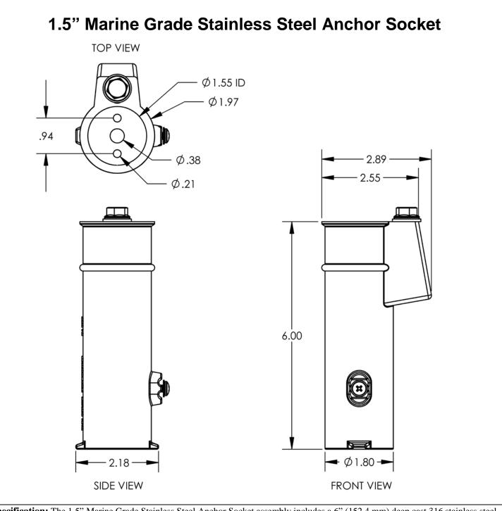
**Specification:** The 1.5" Marine Grade Stainless Steel Anchor Socket assembly includes a 6" (152.4 mm) deep cast 316 stainless steel socket and secures fixtures by means of a bronze wedge assembly. The anchor is intended for moderate to heavy-duty commercial use. It is threaded and comes with a #10 UNC brass grounding screw for bonding. **Shipping Weight:** 1.5 lbs [0.68 kg] (ea)
