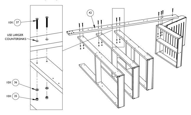
5B. Attach leg (40) to assembly using nuts (35), washers (36), and screws (37). **Do Not Fully Tighten Nuts and Bolts Until Chair is Completely Assembled.**
