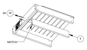
IE. Attach part (6) to assembly with screws (34).
