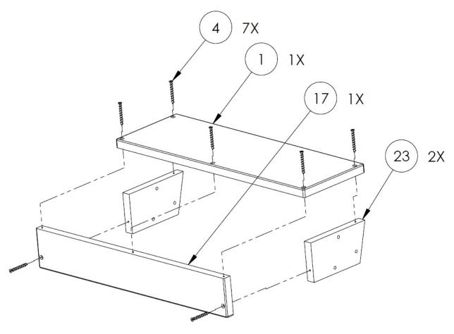
4B. Finished Upper Footrest Assembly should look like the picture below. Next use the 4 assemblies to assemble the chair.
