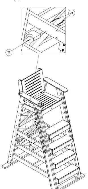
Tighten all fasteners back through assembly to ensure all hardware has been properly tightened.
