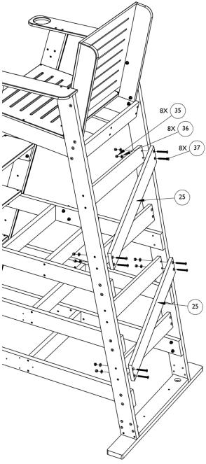
9D. Attach cross braces (26) using nuts (35),
