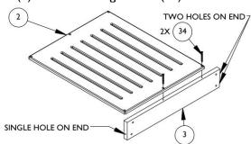
IB. Attach another part (3) to assembly using screws (34).
