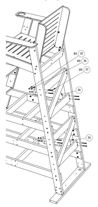
9E. Attach cup holder (27) using screws (34).
