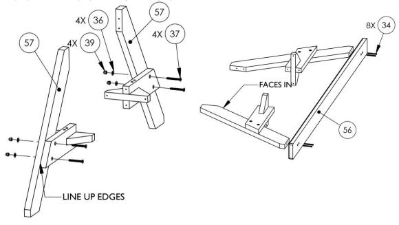
4. Slide support beneath chair. Rotate up so both sides contact the chair.
