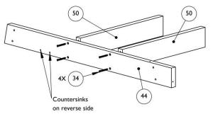
3B. Attach part (45) to 2x part (50) using screws (34).
