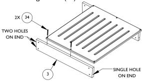
IC. Attach part (4) to assembly with screws (34).
