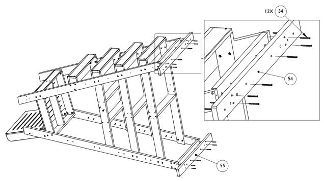
8B. Attach handholds to front base. Use pistol-grip clamps to hold to legs to align.
