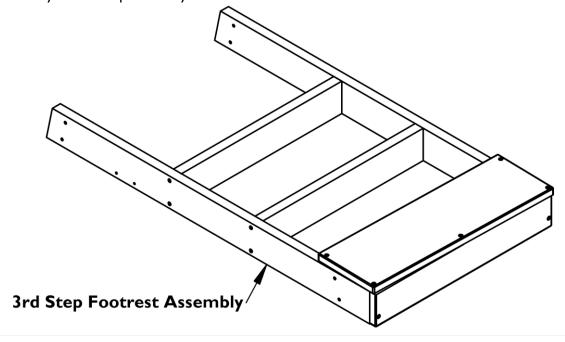
3F. Repeat Steps 3A-3E for the second step assembly using parts (46) and (47) instead of (44) and (45)
