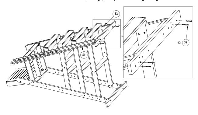
8C. Continue to attach handholds with screws (34) into front legs. Keep pistol-grip clamps in place.
