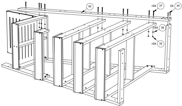
7B. Attach front leg (41) to assembly using bolts (37), screws (34), nuts (36), and washers (35) as shown.
