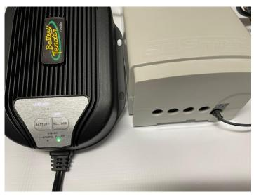
The battery pack should be charged daily. Do not allow battery to fully discharge, as it will shorten battery life. Whenever battery is removed from Control Box or lift that is not in use it is important to connect the battery to the charger. This ensures battery is fully charged and ready for use.
