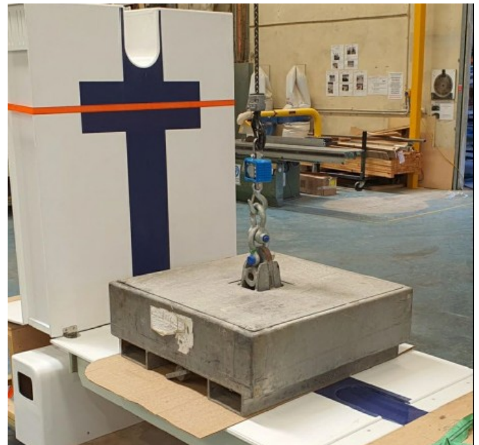
Figure 1. 500kg load cell tests SwimWall skin durability
