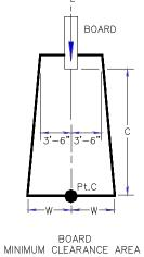
"C" DIMENSION FOR BOARD = AB + BC "W" DIMENSION FOR BOARD = WIDTH AT PT.C
