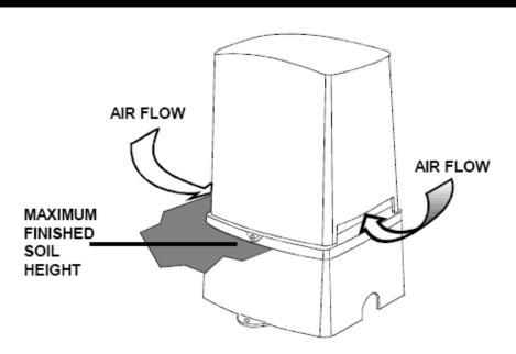
Your 6004 / 6004-AS illuminator needs air to breathe! Lack of ventilation can cause the unit to overheat. This will shorten the lamp life and could damage the unit. DAMAGE TO THE UNIT BECAUSE OF BLOCKED AIR VENTS IS NOT COVERED UNDER OUR WARRANTY!
