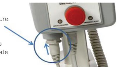
If the lift is not working from the hand controller, unplug the hand controller and try operating the lift from the control box. Does the lift operate?
