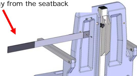
**Figure 2. View of 27" strap orientation on the seatback.**
