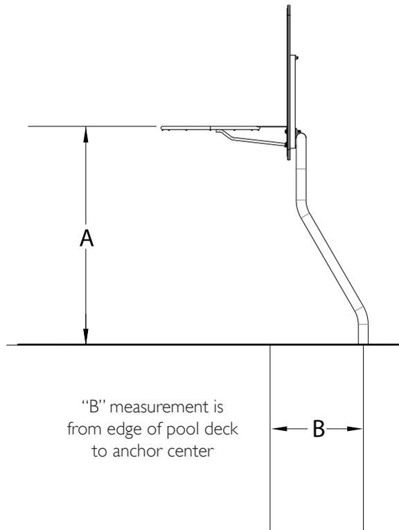
"B" measurement is from edge of pool deck to anchor center
