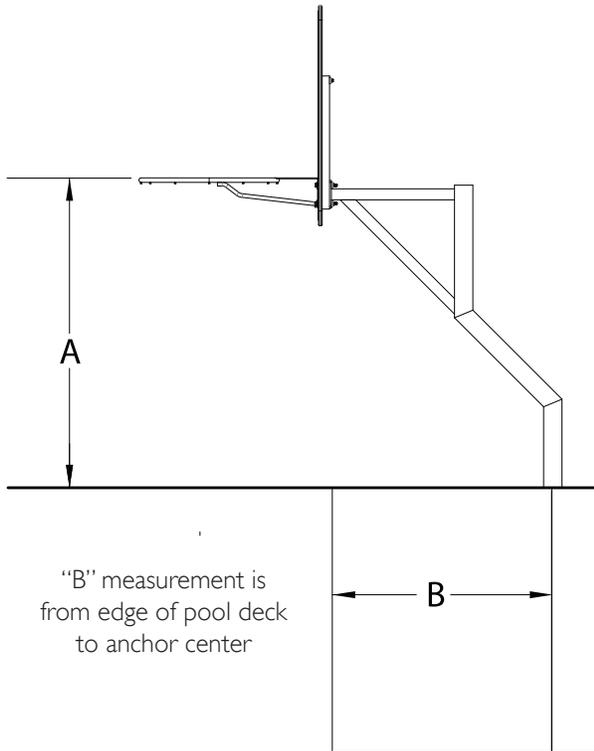
"B" measurement is from edge of pool deck to anchor center
