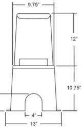
The newly reconfigured LED Star Feature kits now include either a single or dual 12VAC, 5 watt LED light source with a 25- or 50-point fiber optic transmission system for gunite pools or other concrete based features such as patios, walk ways, bar tops, stone/paver walls, etc. These upgraded kits now come in a corrosion resistant, wall- or post-mounted, NEMA 3R enclosure and offer up to 50' fiber runs.
