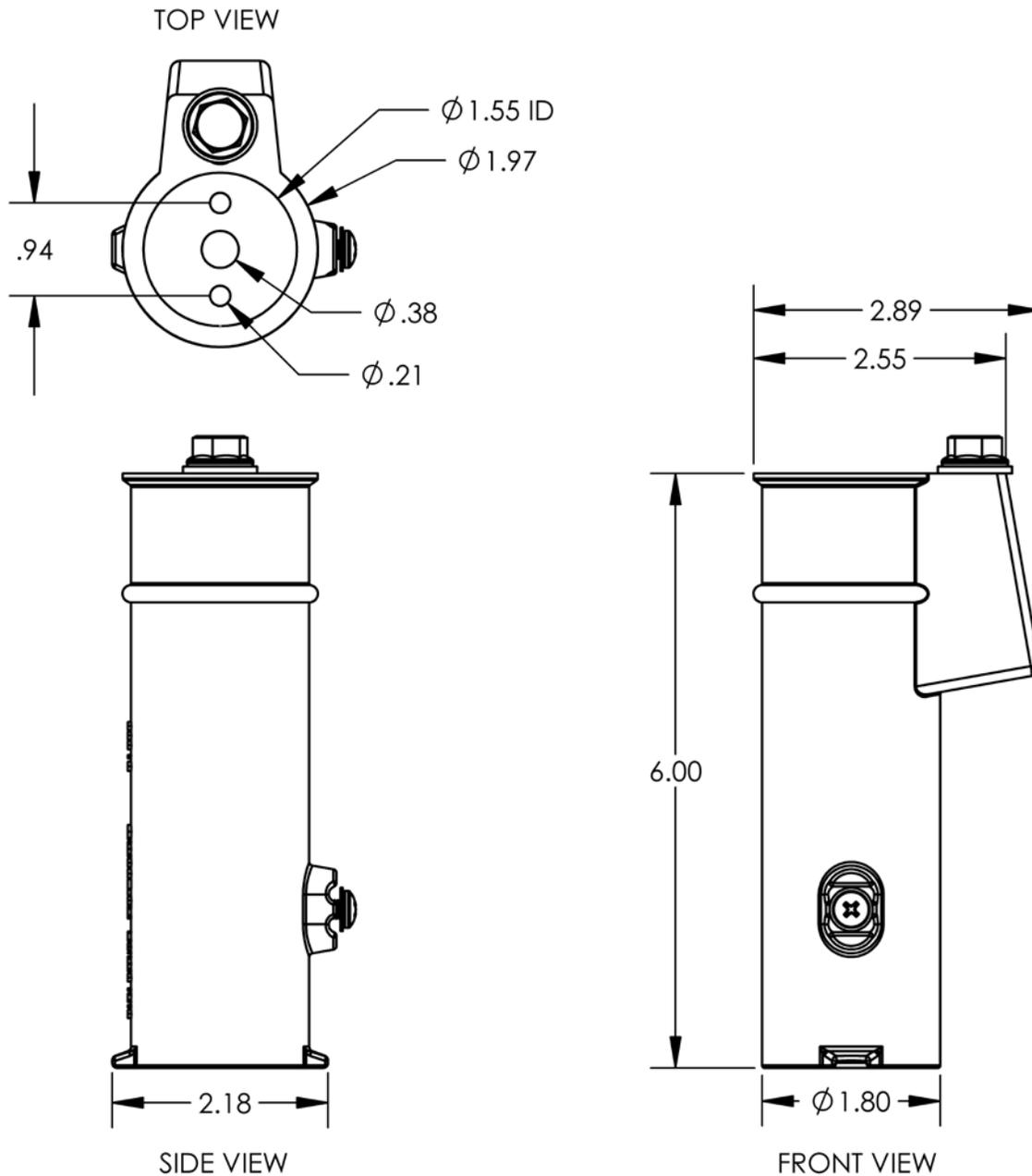
**Specification:** The 1.5" Marine Grade Stainless Steel Anchor Socket assembly includes a 6" (152.4 mm) deep cast 316 stainless steel socket and secures fixtures by means of a bronze wedge assembly. The anchor is intended for moderate to heavy-duty commercial use. It is threaded and comes with a #10 UNC brass grounding screw for bonding.
