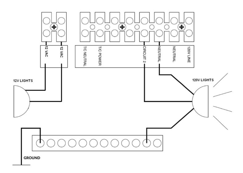
If this product is used to connect 120VAC underwater lights directly, refer to 1999 NEC 680-21(b), 2002 NEC 680-24(b) or CEC 68-060, 062 and 066 for details.
