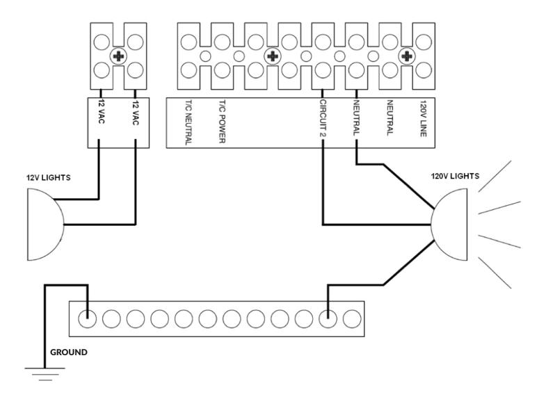
If this product is used to connect 120VAC underwater lights directly, refer to 1999 NEC 680-21(b), 2002 NEC 680-24(b) or CEC 68-060, 062 and 066 for details.
