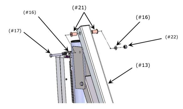
14. Attach the opposite ends of the Actuator Arm Assembly (#12) and Support Arm Assembly (#13) to Seat Bracket with (2) Bolts (#17), (4) Washers (#16) 4) Bushings (#21) and (2) Nuts (#22) in appropriate holes of the Seat Bracket (as shown below), following the same sequence as in previous step.
