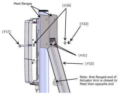
11. Verify that Actuator (#1) is already attached to base of Mast, with (1) Hex Head Bolt (#23), (2) Washers (#16), and (1) Nyloc Nut (#22).
