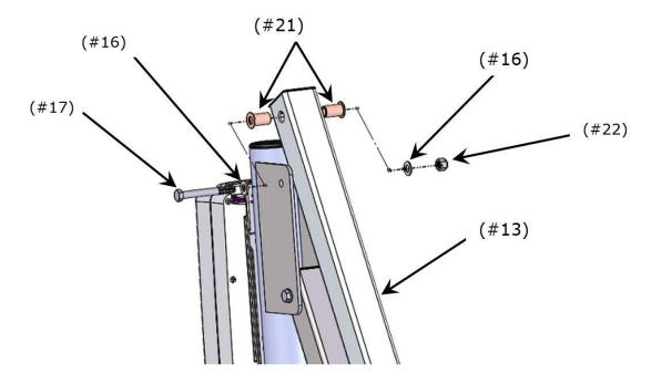
15. Attach the opposite ends of the Actuator Arm Assembly (#12) and Support Arm Assembly (#13) to Seat Bracket with (2) Bolts (#17), (4) Washers (#16) 4) Bushings (#21) and (2) Nuts (#22) in appropriate holes of the Seat Bracket (as shown below), following the same sequence as in previous step.
