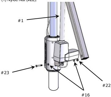
12. Attach the opposite end of the Actuator (#1) to the Actuator Arm Assembly (#12) using (1) Bolt (#23), (2) Washers (#16) and (1) Nut (#22) through the holes in the flanges of the Actuator Arm (see image below).
