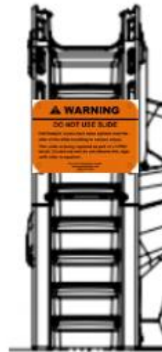
Sign in the correct location
